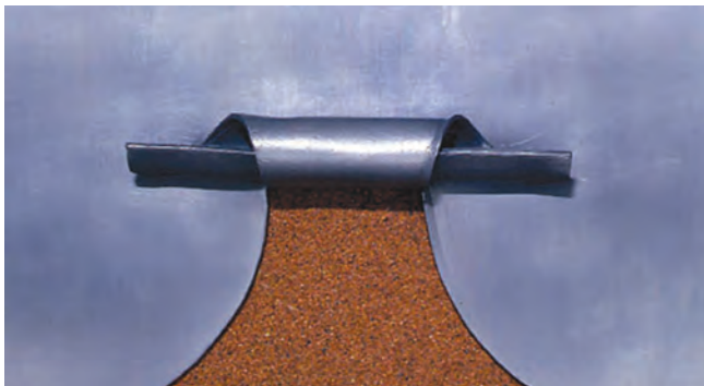
Fig 136. Abutment and sill apron flashing in tile hanging
